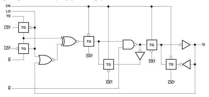
$<sup>\</sup>dagger$  The origins of  $\overline{\text{LD}}$  and  $\overline{\text{CK}}$  are shown in the logic diagram of the overall device.
