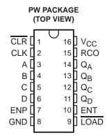
simultaneously so that the outputs change coincident with each other when instructed by the count-enable (ENP, ENT) inputs and internal gating. This mode of operation eliminates the output counting spikes normally associated with synchronous (ripple-clock) counters. A buffered clock (CLK) input triggers the four flip-flops on the rising (positive-going) edge of the clock waveform.
