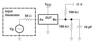
Figure 1. Device Test Setup
