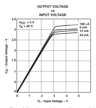
Figure 5. Data Output Voltage vs Data Input Voltage
