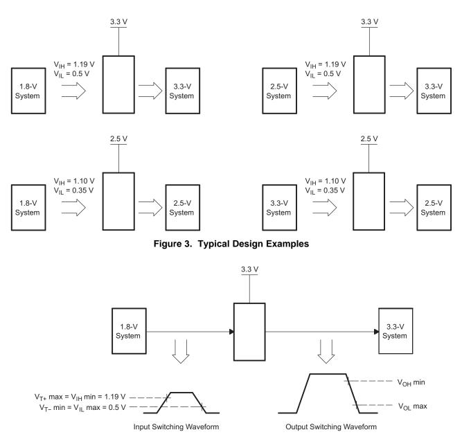
Figure 4. Switching Thresholds for 1.8-V to 3.3-V Translation
