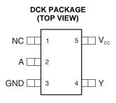
The SN74AUP1T14 performs the Boolean function  $Y = \overline{A}$  with designation for logic-level translation applications with output referenced to supply  $V_{CC}$ .
