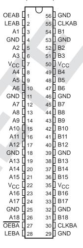
Data flow for B to A is similar to that of A to B but uses  $\overline{\text{OEBA}}$ , LEBA, and CLKBA. The output enables are complementary (OEAB is active high and  $\overline{\text{OEBA}}$  is active low).
