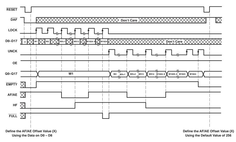
Figure 1. Write, Read, and Flag Timing Reference
