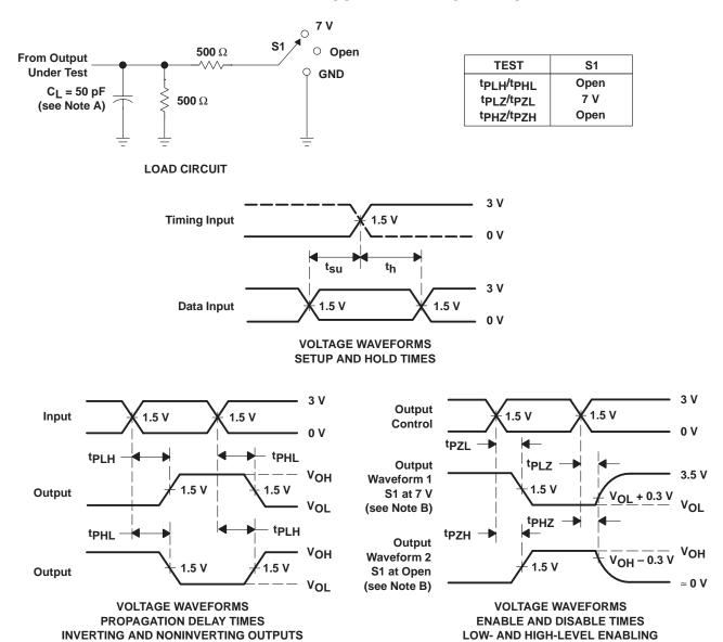
NOTES: A. C<sub>I</sub> includes probe and jig capacitance.
