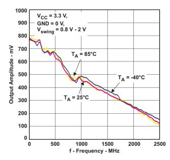
Figure 5. Output Amplitude vs. Frequency
