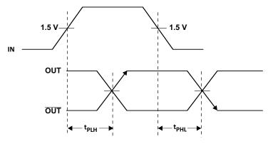
Figure 2. Output Propagation Delay
