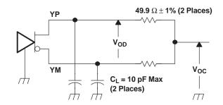
NOTE A: The lumped instrumentation capacitance for any single-ended voltage measurement is less than or equal to 10 pF. When making measurements at YP or YM, the complementary output is similarly loaded.
