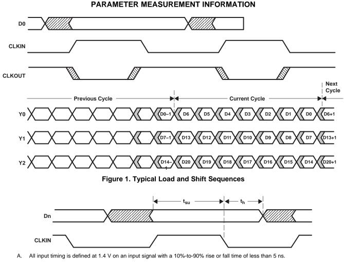
Figure 2. Setup and Hold Time Definition
