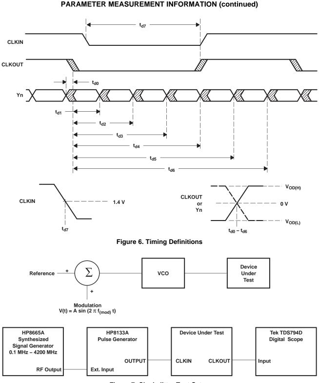
Figure 7. Clock Jitter Test Setup
