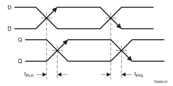
Figure 2. Propagation Delay
