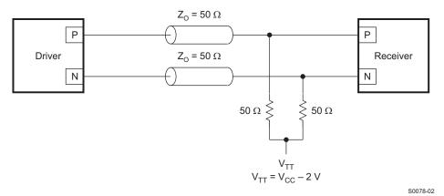
Figure 1. Typical Termination for Output Driver
