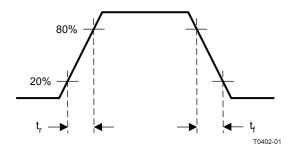
Figure 4. Output Rise and Fall Times
