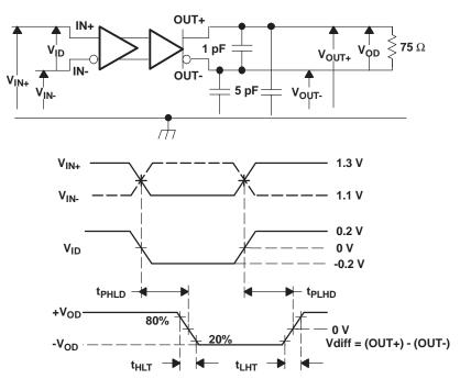
NOTE: All input pulses are supplied by a generator having the following characteristics: t<sub>r</sub> or t<sub>f</sub> ≤ .25 ns, pulse-repetition rate (PRR) = 0.5 Mpps, pulse width = 500 ± 10 ns. C<sub>L</sub> includes instrumentation and fixture capacitance within 0,06 mm of the D.U.T.
