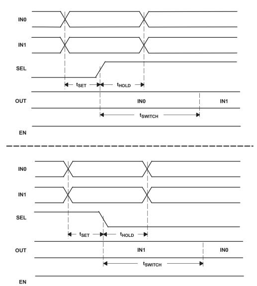
NOTE: t<sub>SET</sub> and t<sub>HOLD</sub> times specify that data must be in a stable state before and after mux control switches.
