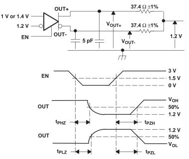
NOTE: All input pulses are supplied by a generator having the following characteristics: t<sub>r</sub> or t<sub>f</sub> ≤ 1 ns, pulse-repetition rate (PRR) = 0.5 Mpps, pulse width = 500 ± 10 ns. C<sub>L</sub> includes instrumentation and fixture capacitance within 0,06 mm of the D.U.T.
