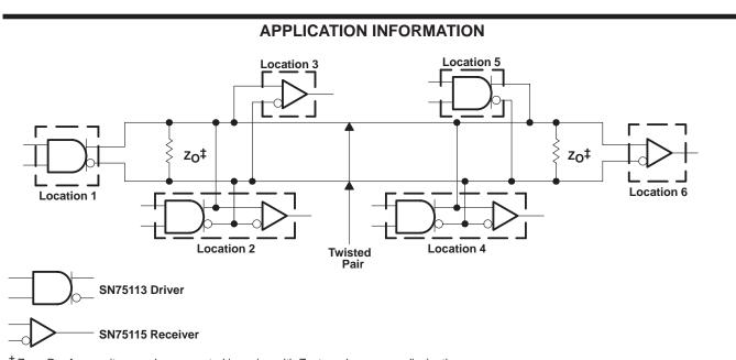
$\ddagger$  Z<sub>O</sub> = R<sub>T</sub>. A capacitor may be connected in series with Z<sub>O</sub> to reduce power dissipation.
