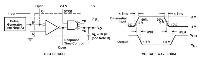
NOTES: A. The pulse generator has the following characteristics:  $Z_O$  = 50  $\Omega$ , PRR  $\leq$  500 kHz,  $t_W \leq$  100 ns, duty cycle = 50%.
