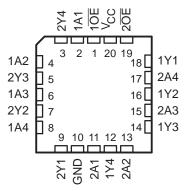
These devices are organized as two 4-bit line drivers with separate output-enable  $(\overline{OE})$  inputs. When  $\overline{OE}$  is low, the device passes data from the A inputs to the Y outputs. When  $\overline{OE}$  is high, the outputs are in the high-impedance state.
