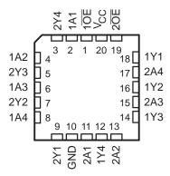
These devices are organized as two 4-bit line drivers with separate output-enable  $(\overline{OE})$  inputs. When  $\overline{OE}$  is low, the device passes data from the A inputs to the Y outputs. When  $\overline{OE}$  is high, the outputs are in the high-impedance state.
