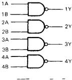
$Y = \overline{A \cdot B}$  or  $Y = \overline{A} + \overline{8}$
