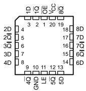
To ensure the high-impedance state during power up or power down,  $\overline{OE}$  should be tied to V<sub>CC</sub> through a pullup resistor; the minimum value of the resistor is determined by the current-sinking capability of the driver.
