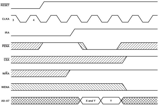
Figure 9. Programming X and Y Separately for AF/AEA
