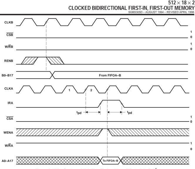
Figure 5. Write-Cycle and IRA-Flag Timing When FIFOA-B Is Full<sup>†</sup>
