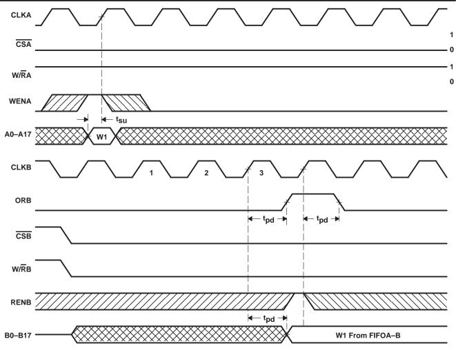
Figure 4. ORB-Flag Timing and First Data-Word Fall-Through When FIFOA-B Is Empty<sup>†</sup>
