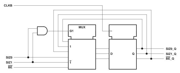
Figure 2. Logic Diagram for SIZ0, SIZ1, and BE Register
