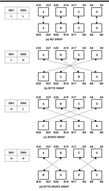
Figure 3. Byte Swapping (Long-Word Size Example)
