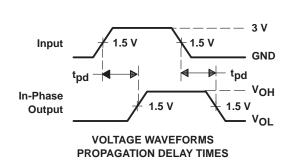
NOTES: A. Includes probe and jig capacitance
