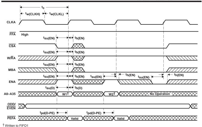
Figure 5. Port-A Write Cycle for FIFO1
