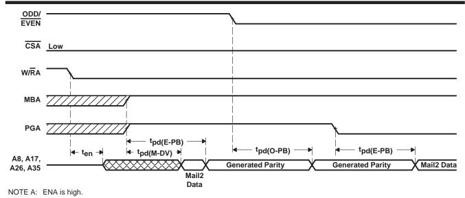
Figure 25. Parity-Generation Timing When Reading From the Mail2 Register
