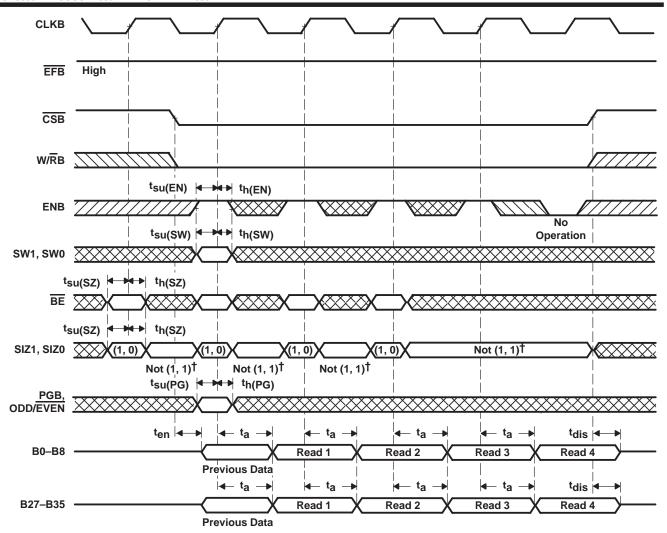
† SIZ0 = H and SIZ1 = H selects the mail1 register for output on B0–B35. NOTE A: Unused bytes hold last FIFO1 output register data for byte-size reads.
