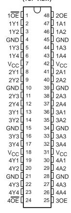
These devices can be used as four 4-bit buffers, two 8-bit buffers, or one 16-bit buffer. These devices provide true outputs and complementary output-enable (OE and  $\overline{OE}$ ) inputs.
