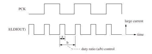
The intermittent current output from LDIOUT is automatically adjusted as the frequency changes to maintain the duty ratio almost constant. The intermittent current duty ratio is set by resistor  $R_{DUTY}$  connected between DUTY and VSS pins, and is given by the following equation.
