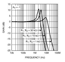
Figure 48. Closed Loop Frequency Response
