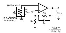
Figure 52. Thermopile Sensor Interface
