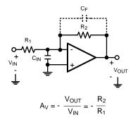
Figure 47. Compensating for Input Capacitance
