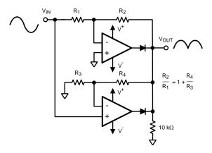
Figure 53. Precision Rectifier
