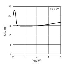
Figure 46. Input Common Mode Capacitance
