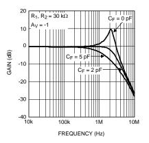
Figure 49. Closed Loop Frequency Response
