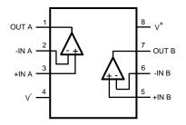
Figure 3. 8-Pin VSSOP – Top View See Package Number DGK
