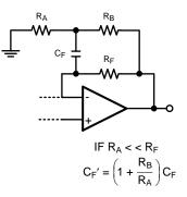
Figure 51. Modified Transimpedance Amplifier
