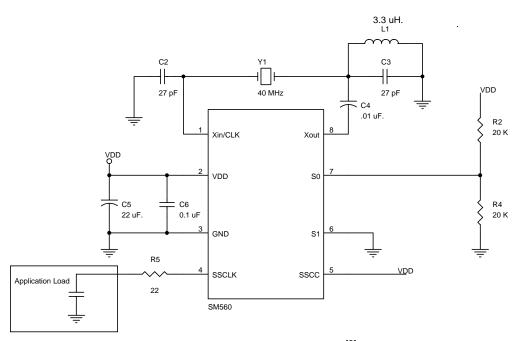
Figure 3. Application Schematic<sup>[2]</sup>
