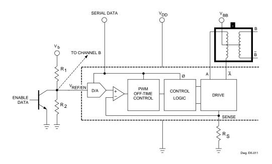
FIGURE 2. PWM CONTROL (RUN MODE)
