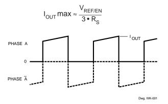
FIGURE 1. PHASE A COIL CURRENT WAVEFORM
