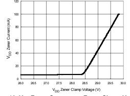
Figure 19. V<sub>DD</sub> Zener Current vs. Zener Clamp Voltage
