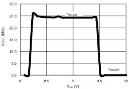
Figure 16. Green-Mode Burst Back and Green-Mode Off Frequency vs. V<sub>DD</sub>
