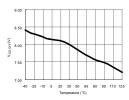
Figure 8. Turn-off Threshold Voltage (V<sub>DD-OFF</sub>) vs. Temperature
