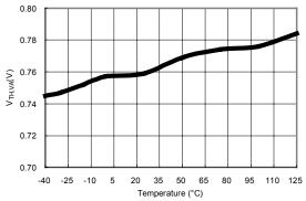
Figure 14. Valley Threshold Voltage (VSTHVA) vs. Temperature
