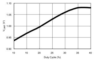
Figure 18. VLIMIT Ramp vs. Duty Cycle
