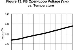
Figure 15. Output Voltage Low (VGATE-L) vs. Temperature
