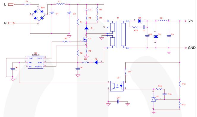
Figure 21. Reference Circuit (with Secondary-Side Feedback)
