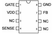
Figure 5. DIP-8 Pin Configuration
