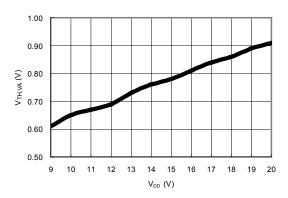
Figure 17. Valley Threshold Voltage (V<sub>STHVA</sub>) vs. V<sub>DD</sub>
