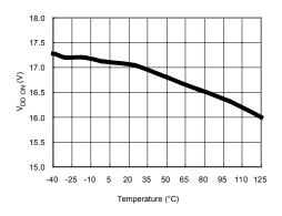
Figure 7. Turn-on Threshold Voltage (V<sub>DD-ON</sub>) vs. Temperature
