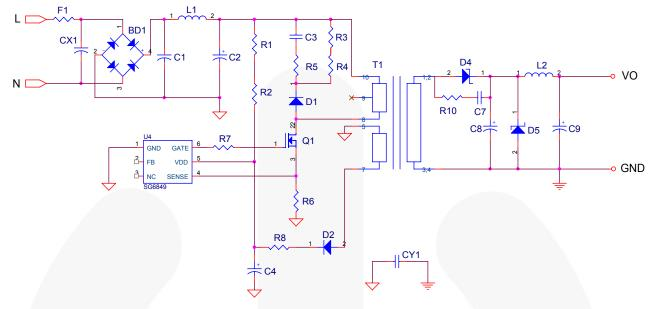
Figure 20. Reference Circuit (without Secondary-Side Feedback)
