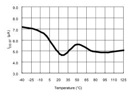
Figure 9. Startup Current (I<sub>DD-ST</sub>) vs. Temperature
