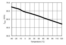
Figure 11. Center Frequency (fosc) vs. Temperature
