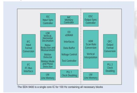
The SDA 9400 contains all necessary functional blocks on a single chip:
