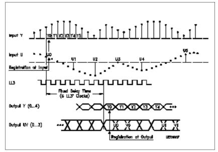
Signal Delay Time for U, V and Y (used indication: number of scanning values).
