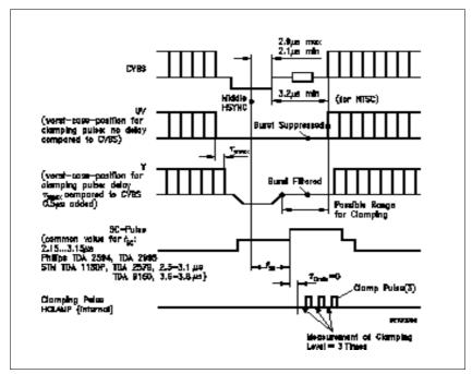
**Clamping Pulse Timing**
