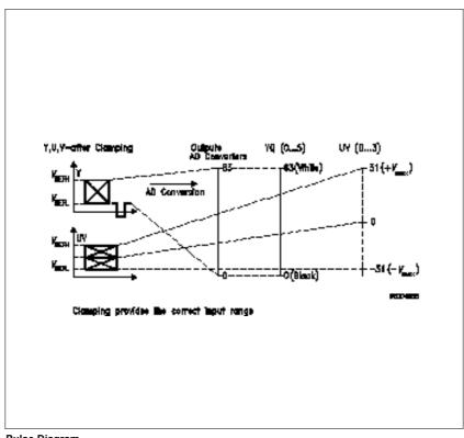
Pulse Diagram Input Voltage Range of Y, U, and V and their Translation in Initial Values ('Digital Values')
