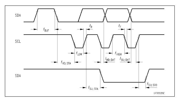
Figure 2 Timing Conditions for the  ${\rm I}^2{\rm C}$  Bus (high-speed mode)
