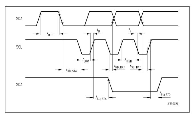
Figure 2 Timing Conditions for the  ${\rm I}^2{\rm C}$  Bus (high-speed mode)
