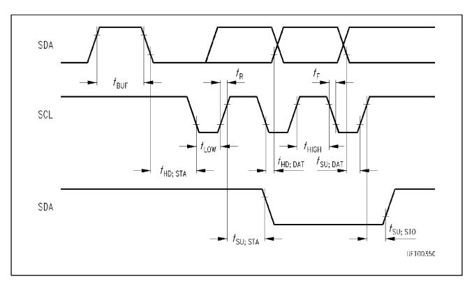
Figure 2 Timing Conditions for the  $I^2C$  Bus (high-speed mode)
