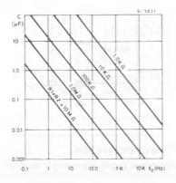
The charge time (output HIGH) is given by t<sub>1</sub> = 0.693 (R1 + R2) C1
