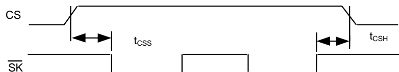
Figure 4 Timing Chart for t_{CSS} and t_{CSH} when \overline{SK} is "H"
