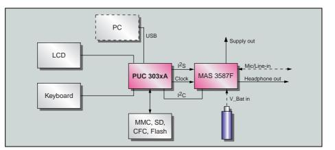
Fig. 1: Typical application: multistandard audio secure player/recorder
