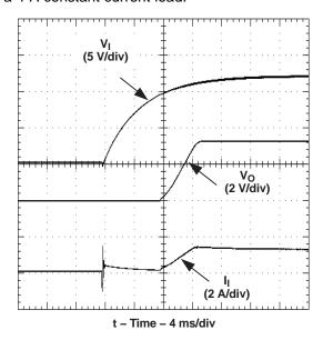
Figure 12. Power-Up Waveforms
