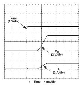
Figure 14. Power Up Response From Inhibit Control
