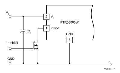
Figure 13. On/Off Inhibit Control Circuit
