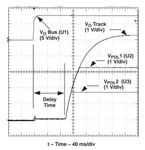
Figure 9. AutoTrack™ Control Waveform
