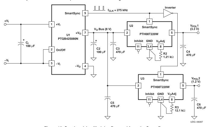
Figure 10. Synchronizing Modules Powered from the Same Bus
