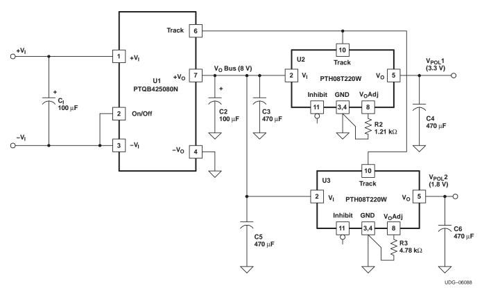
Figure 8. Power-Up Sequencing Using AutoTrack™ Control
