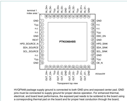
thermal vias need to be incorporated in the PCB in the thermal pad region.
