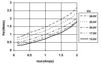
Note 1: All data listed in the above graphs, except for derating data, has been developed from actual products tested at 25°C. This data is considered typical data for the ISR. Note 2: Minimum V<sub>in</sub> data is typical and is not guaranteed. The data corresponds to a 2% output voltage drop. Note 3: Thermal derating graphs are developed in free air convection cooling of 40-60 LFM with no optional heat tab. (See Thermal Application Notes). www.ti.com
