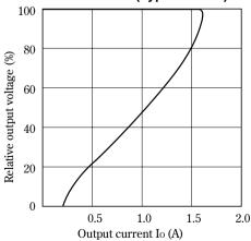
Fig. 5 Output Voltage Adjustment Characteristics
