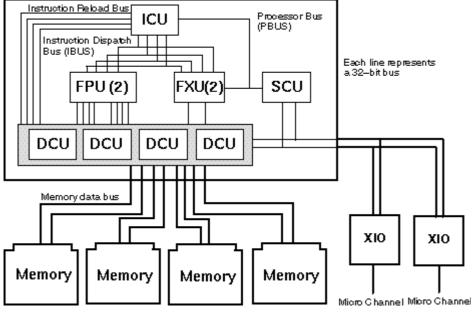
ICU Instruction Cache Unit FXU Fixed Point Unit FPU Floating Point Unit DCU Data Cache Unit SCU Sorage Control Unit
