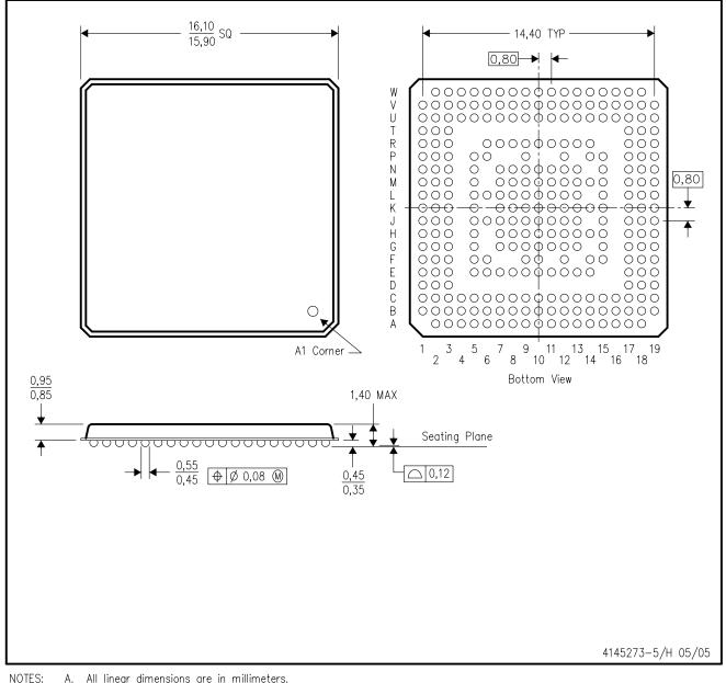
A. All linear dimensions are in millimeters.
