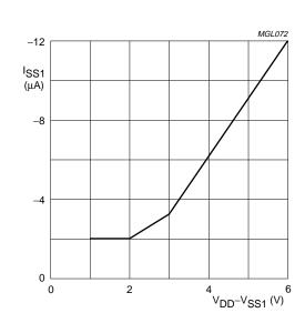
Fig.11 Typical supply current ( $I_{SS1}$ ) as a function of clock supply voltage ( $V_{DD} - V_{SS1}$ ) at  $T_{amb} = -40$  to +85 °C.
