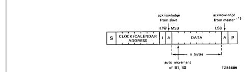
(1) The master receiver must signal an end of data to the slave transmitter by **not** generating an acknowledge on the **last byte** that has been clocked out of the slave.
