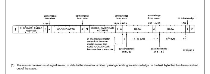
Fig.9 Master transmitter reads clock/calendar after setting mode pointer.
