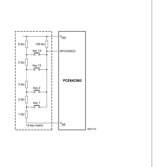
Fig.14 A typical ADC application for keypad detection.
