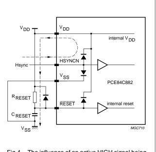
Fig.4 The influence of an active HIGH signal being applied before Power-on-reset.
