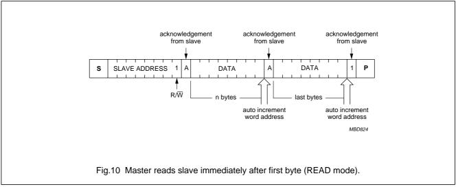
An unlimited number of data bytes can be read in one operation. The address is automatically incremented. If a read without setting the word address is performed after a write operation, the address pointer may point at a byte in the row after the previously written row. This occurs if, during writing, the three lowest address bits (column) rolled over.
