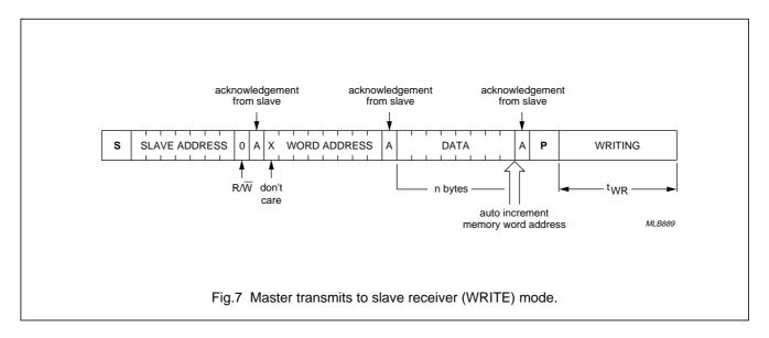
After the word address, one-to-eight data bytes can be sent. The address is automatically incremented, but the four highest address bits (row) are internally latched. Therefore all bytes are written in the same row.
