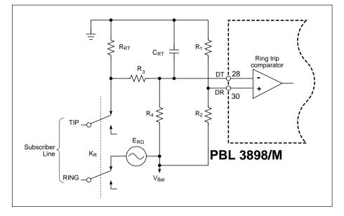
Figure 21. Ring trip network, unbalanced ringing.
