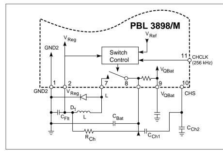
Figure 18. Switch mode regulator.
