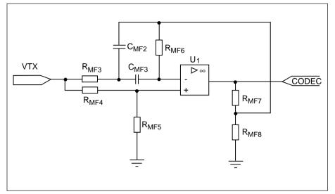
Figure. 23. Metering notch filter
