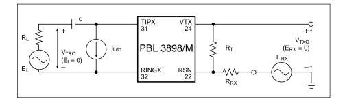
Figure 2. Overload level.  $1/\omega C \ll R_L, R_L = 600 \text{ ohm},$  $R_\tau = 30,6 \text{ kohms}, R_{R_X} = 30 \text{ kohms}.$
