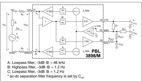
Figure 13. Simplified ac transmission circuit.
