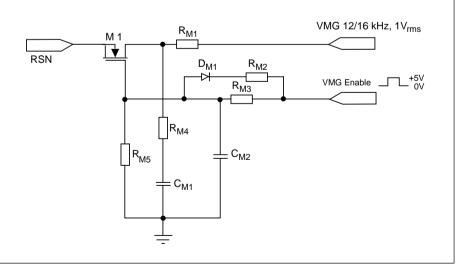
Figure 22. Metering injection circuit.
