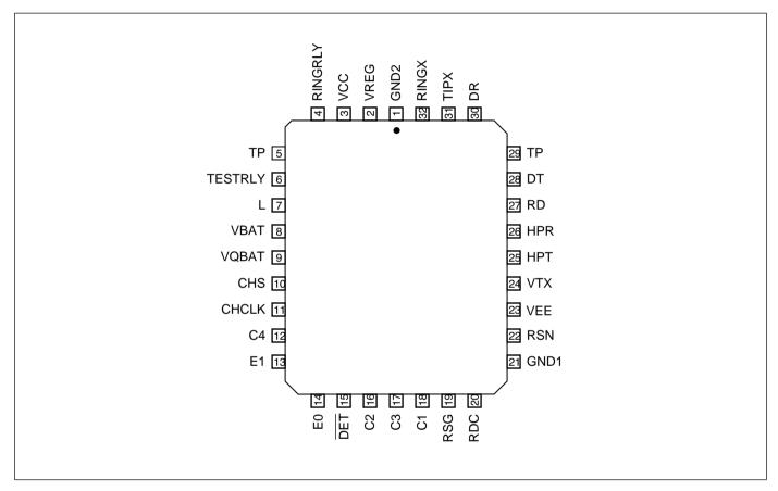
Figure 11. Pin configuration, 32-pin j-leaded chip carrier, Top view.
