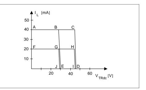
The open circuit voltage is then, for a programmed loop current of 40mA, 29.5V for  $R_{sc}$  = open circuit and 45.8 V for  $R_{sc}$  = 0.
