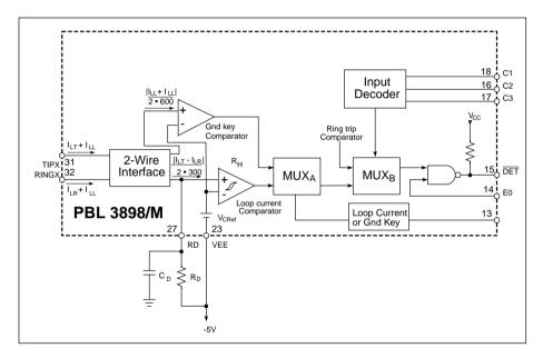
Figure 19. Loop current and ground key detector.
