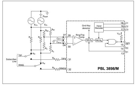
Figure 20. Ring trip network, balanced ringing.
