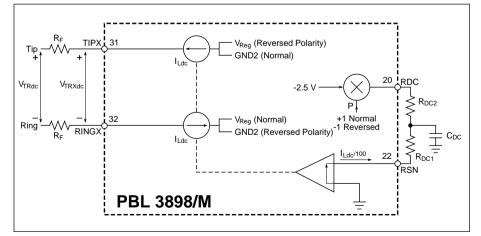
Figure 16. Battery feed.
