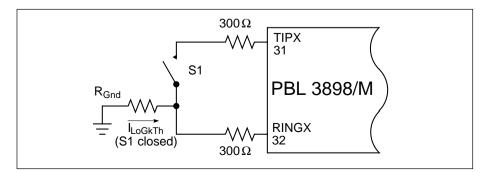
Figure 10. Ground key detector.
