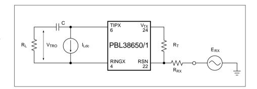
Figure 3. Longitudinal to metallic ( $B_{\rm LME}$ ) and Longitudinal to four-wire ( $B_{\rm LFE}$ ) balance
