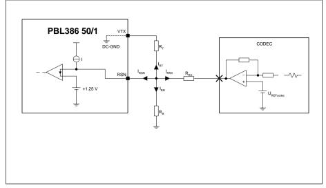
Figure 14. CODEC receive interface.
