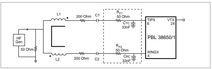
Figure 8. RFI Test Circuit.
