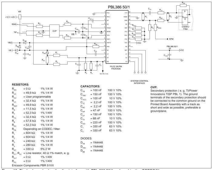
Figure 12. Single-channel subscriber line interface with PBL 386 50/1 and combination CODEC/filter.
