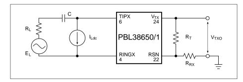
Figure 5. Overload level,  $V_{\rm TXO}$ , four-wire transmit port
