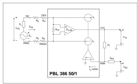
Figure 10. Simplified ac transmission circuit.
