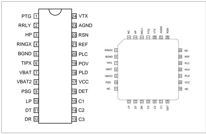
Figure 9. Pin configuration, 24-pin SOIC and 28 pin PLCC package, top view.
