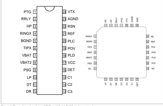
Figure 8. Pin configuration, 24-pin SOIC and 28 pin PLCC package, top view.
