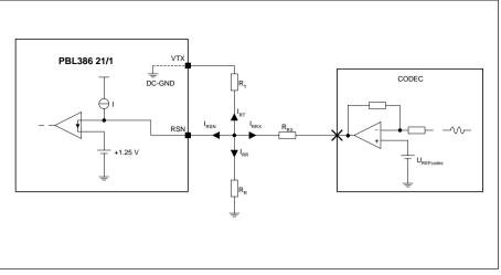
Figure 13. CODEC receive interface.
