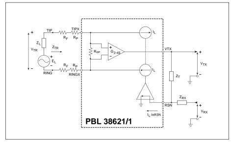
Figure 9. Simplified ac transmission circuit.
