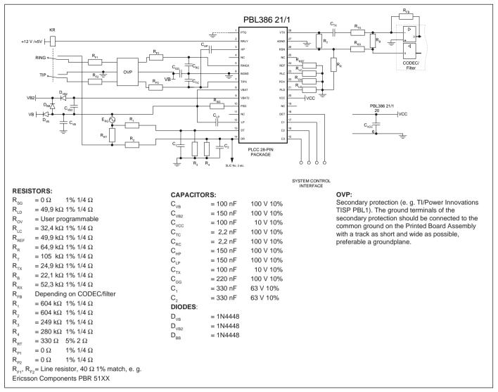
Figure 11. single-channel subscriber line interface with PBL 386 21/1 and combination CODEC/filter.
