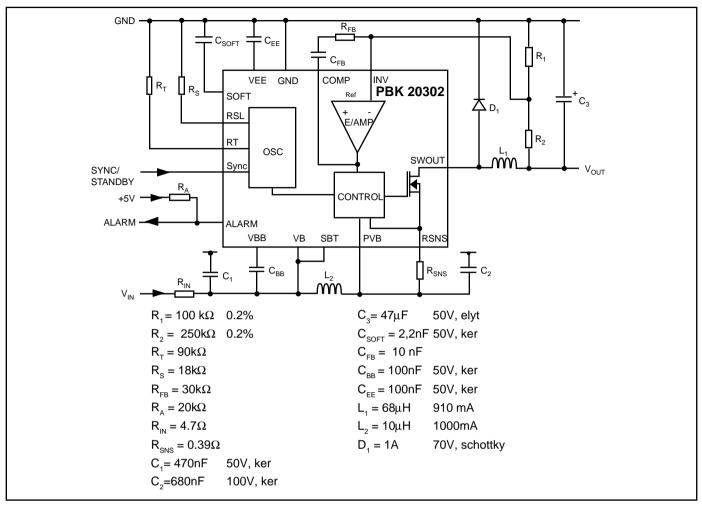
Figure 4. Typical step-down converter application.
