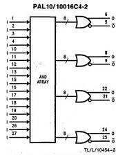
$V_{EE}=\cdot 14,\,V_{CC}=28,\,V_{CC0}\,(5,\,6,\,8,\,9)=7,\\ V_{CC0}\,(21,\,22,\,24,\,25)=23$  Pinout applies to 28-pin PLCC
