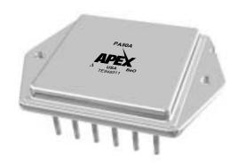
The JEDEC MO-127 12-pin Power Dip™ package (see Package Outlines) is hermetically sealed and isolated from the internal circuits. The use of compressible thermal washers and/or improper mounting torque will void the product warranty. Please see "General Operating Considerations".
