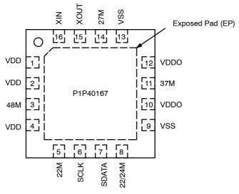
Figure 2. Pin Configuration (Top View)
