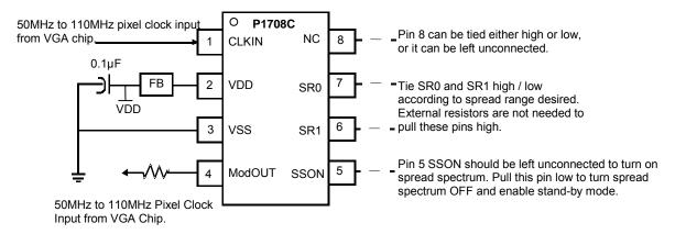
Note: To set the P1708C to standby mode, disable the input clock (pin 1 CLKIN) and pull SSON (pin 5) low. Refer to Standby Mode Selection Table.
