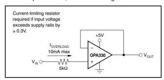
Figure 18. Input Current Protection
