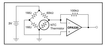
Figure 23. Thermistor Measurement
