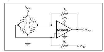
Figure 21. Single Op Amp Bridge Amplifier
