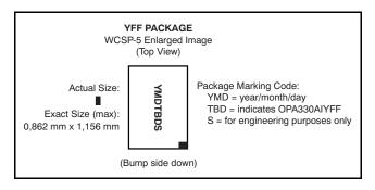
Figure 25. YFF Package Marking
