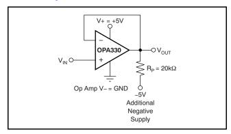
Figure 20. For V<sub>OUT</sub> Range to Ground
