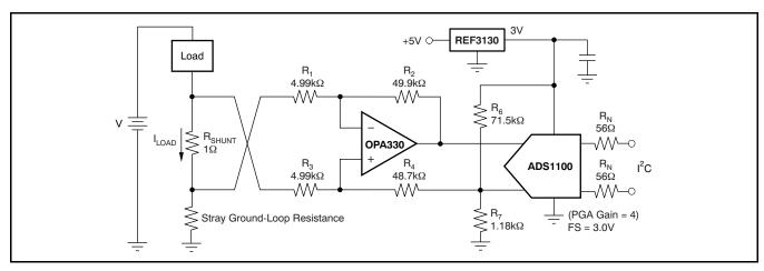
NOTE: 1% resistors provide adequate common-mode rejection at small ground-loop errors.
