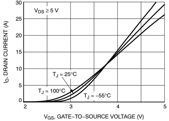
Figure 2. Transfer Characteristics
